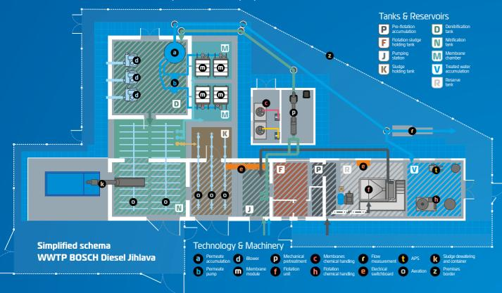
The tanks of the smaller line were roofed and partially turned into a new physical-chemical pretreatment technology for industrial wastewaters. Atop the roof a new building for a flotation unit was built. The flotation unit was not a part of the original WWTP, the industrial wastewaters were treated in a flotation unit in the factory area. The new WWTP further contains a new assembled building for a mechanical screen and chemical handling.
