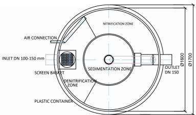
Note: Drawing of WWTP for backfill or concreeting. Assembly make according to the Instruction for installation. \* In case the WWTP has to be instaled deeper than maximal allowed dimension (see the drawing) or the soil load around the WWTP or underground water level i higher then we strongly recommend statically secure the WWTP tank (e.g. concreeting).
