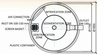
Note: Drawing of WWTP for backfill or concreeting. Assembly make according to the Instruction for installation. \* In case the WWTP has to be instaled deeper than maximal allowed dimension (see the drawing) or the soil load around the WWTP or underground water level i higher then we strongly recommend statically secure the WWTP tank (e.g. concreeting).
