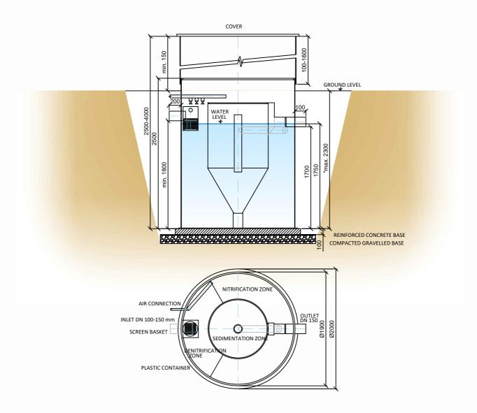
Note: Drawing of WWTP for backfill or concreeting. Assembly make according to the Instruction for installation.
