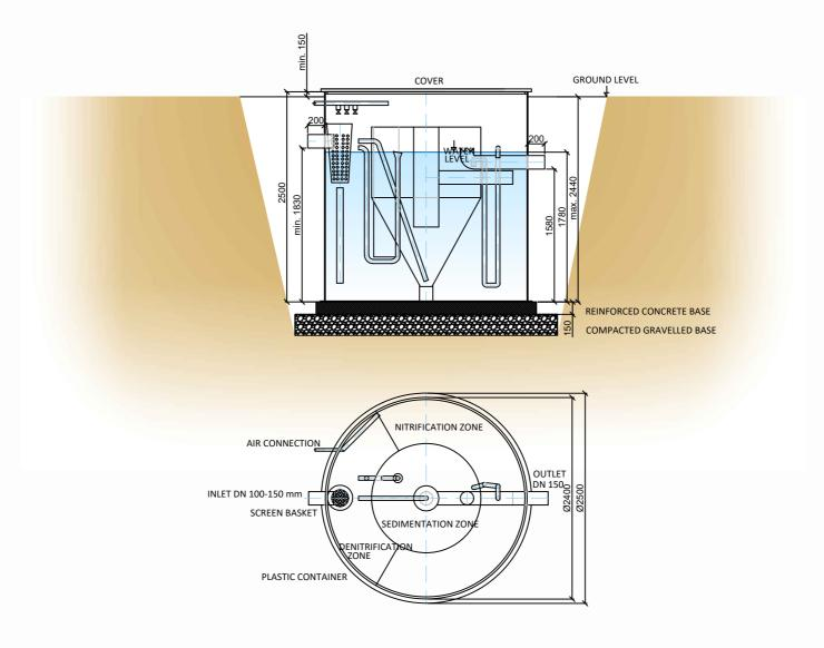
Note: Drawing of WWTP for backfill or concreeting. Assembly make according to the Instruction for installation. \* In case the WWTP has to be instaled deeper than maximal allowed dimension (see the drawing) or the soil load around the WWTP or underground water level i higher then we strongly recommend statically secure the WWTP tank (e.g. concreeting).
