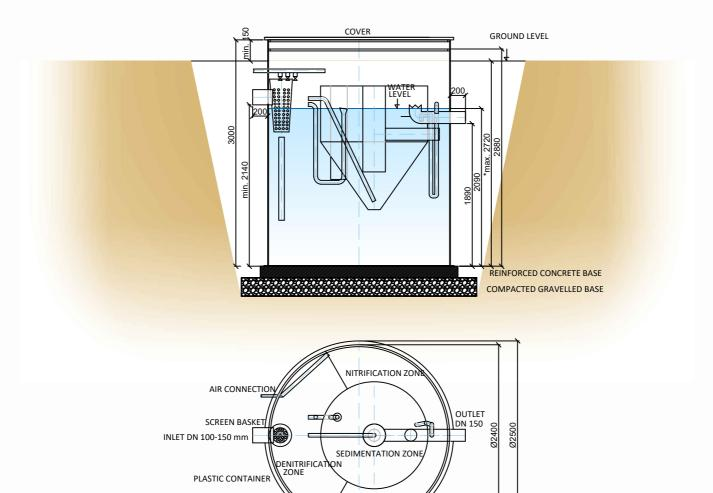
Note: Drawing of WWTP for backfill or concreeting. Assembly make according to the Instruction for installation. \* In case the WWTP has to be instaled deeper than maximal allowed dimension (see the drawing) or the soil load around the WWTP or underground water level i higher then we strongly recommend statically secure the WWTP tank (e.g. concreeting).
